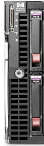
As the world's most popular blade server, the HP ProLiant BL460c Server Blade sets the standard for the data center. Packing two processors, two hot plug hard drives, up to 192GB of memory, and a dual-port 10 gigabit Ethernet adapter into a half-height blade, the BL460c gives IT managers the performance and expandability they need for demanding data center applications.
